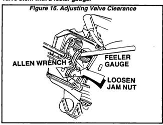
4. When valve clearance is correct, hold the pivot ball stud with the allen wrench while tightening the rocker arm jam nut with a crow's foot. Tighten the jam nut to the specified torque. After tightening the jam nut, recheck the valve clearance to make sure it did not change.
